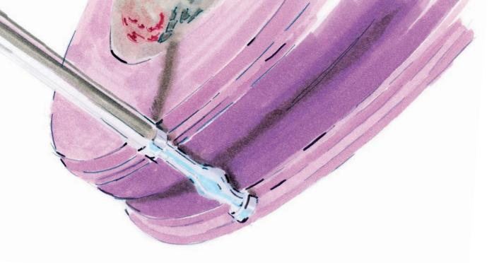
**Roll grinding** is a process that involves intensive levels of grinding. Different rollers made from very differ-ent materials and in different sizes always require the right wheel. What remains the same, however, is the defined surface quality that you will achieve using our tools. Our ceramic-bonded CBN wheels are often a more economical alternative for roll grinding.
