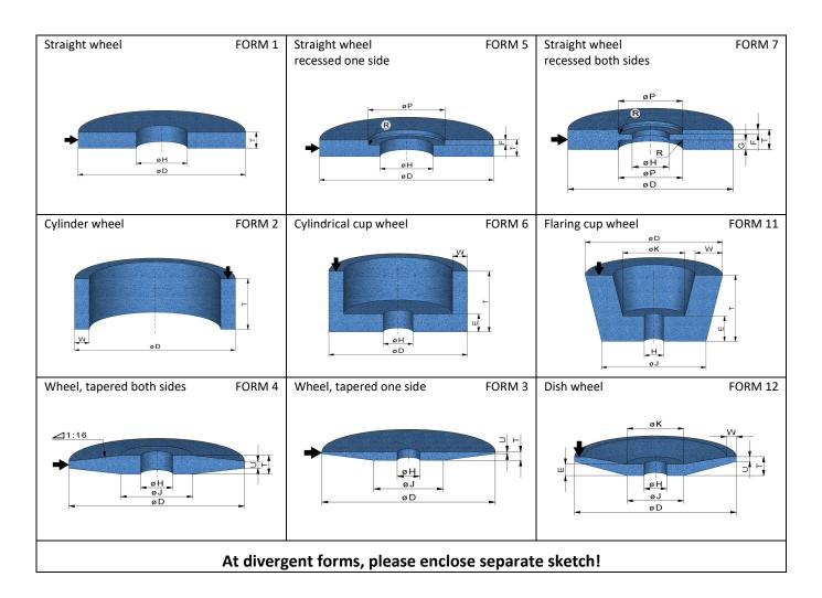
Straight grinding wheels can be provided with different profiles. The profiles are named with letters and have the following meaning:
